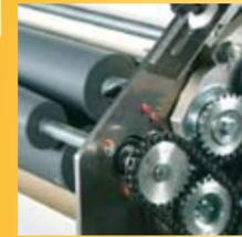
The drivers and adjusting devices for the belts and rolling cylinders are of a particularly robust construction, and supported by aluminium sidewalls milled from the block. The feeding cylinder which is shaped like a spindle and the non-deforming belt ensure both accuracy and conformity in the finished products.
