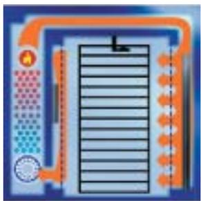
Effectively insulated ovens mean economic baking. The oven walls contain 100-mm thickness of overlapping Rockwool® plus a 20-mm void. The roof insulation is 150 mm thick.
