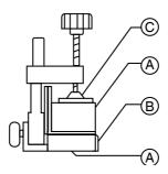
When cut the Al extrusion product(B), can use the block(A) or other block in order to avoid the work piece deformation. At same time to use cutting oil and prevent the AL fragment accumulation near to the blade.
