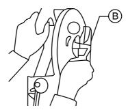
6) To assemble the blade, confirm the arrow direction is coincident between the blade and guard (figure 5).
