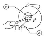
5) press down the lock of shaft(A) and the blade can't turn round, to loose the screw bolt of blade with wrench(B) turn clockwise then to take off the screw, external pressure plate and blade(figure 4)
