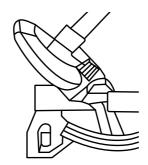
12) To loose the lock of miter(A), Lean the arm to left, when the indictor(B) point to right angle on the scale(C), to tighten the lock of miter(A) (figure 13)
