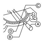
To loose the handle(A) with anticlockwise, To rotary the table at same time press down position lock(B), When the indicator(C) point to right angle on the scale(D), to tighten the handle(A) with clockwise.
